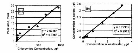
Figure 2. Calibration curves for (a) HPLC peak area versus *chlorpyrifos* concentration, (b) *chlorpyrifos* concentration in extract versus *chlorpyrifos* concentration in wastewater
